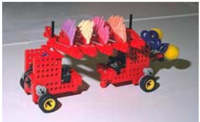
Figure 3. Creature with two built-in Crickets, which communicate with one another to synchronize their motion
