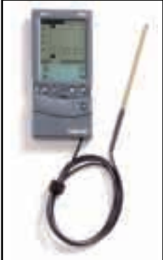
Figure 1. ImagiProbe setup: PalmPilot, D/A converter, probe.
