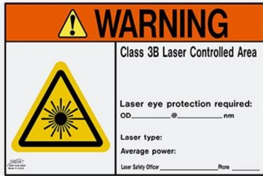
Figure 6a: Sample ANSI Z535.2 compliant warning sign for Class 3B laser controlled areas. Laser Safety Industries, 2016
