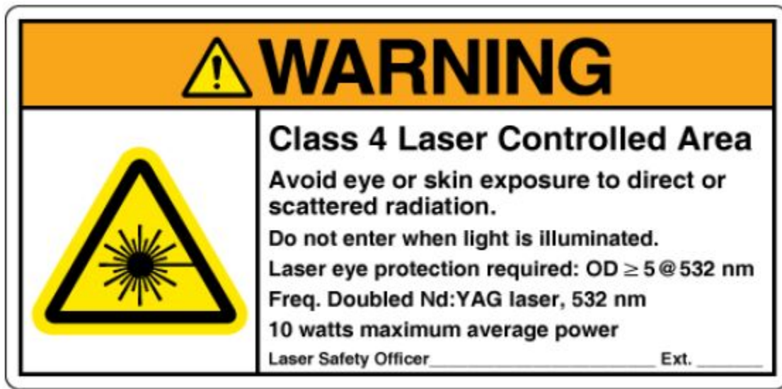
Figure 6b: Sample ANSI Z535.2 compliant warning sign for Class 3B and Class 4 laser controlled areas. ANSI Laser Safety Standard, 2014
