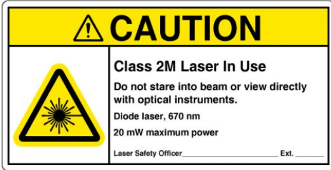
Figure 5: Sample ANSI Z535.2 compliant warning sign for Class 2, Class 2M, and Class 3R lasers. ANSI Laser Safety Standard, 2014
