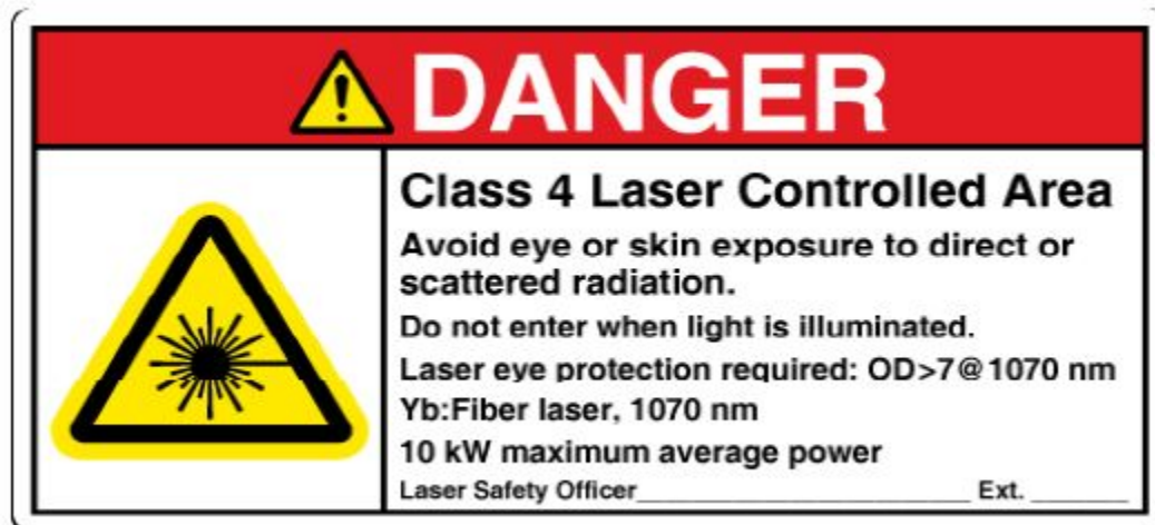
Figure 7: Sample ANSI Z535.2 compliant Class 4 laser controlled area danger sign format. ANSI Laser Safety Standard, 2014
