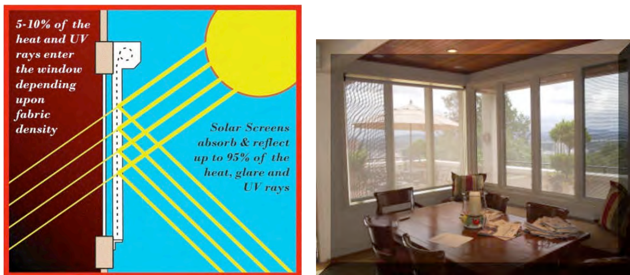
Figure 56. A solar screen blocks heat from hitting window glass (left), but does not block the view from inside the building (right) 389
