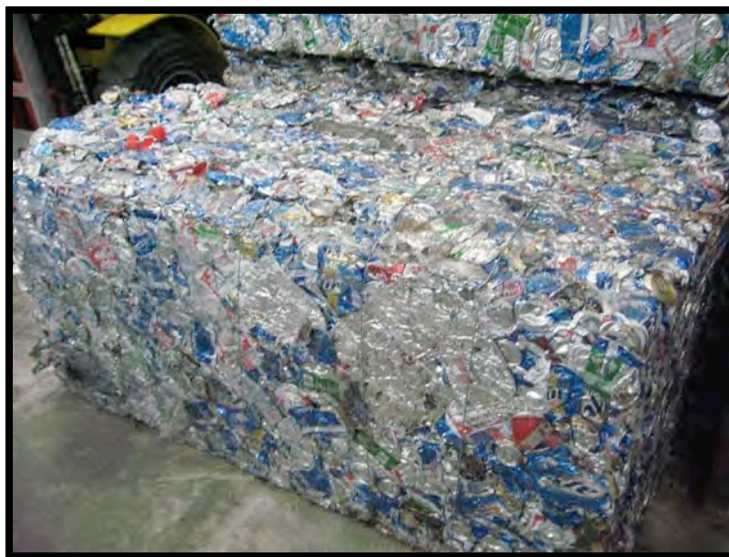
Figure 3.8: Metal shipped for recycling is weighed and shipped in bales.
