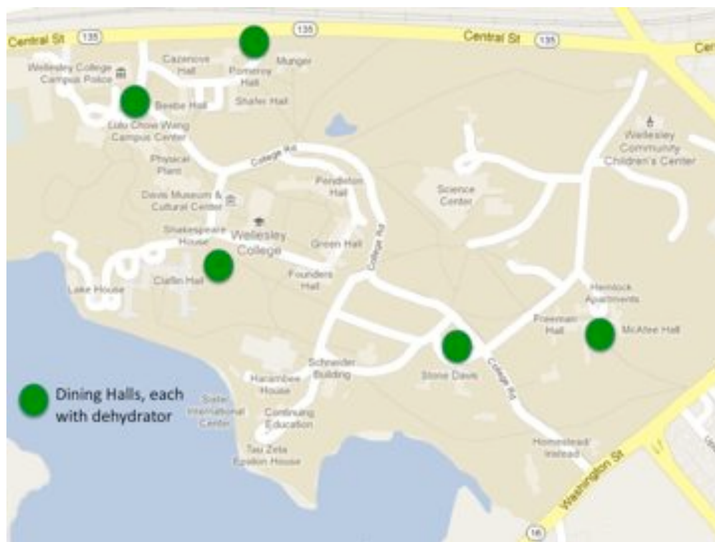
Figure 13-2. Decentralized model for on-campus dehydration. One ECORECT unit in each dining hall.
